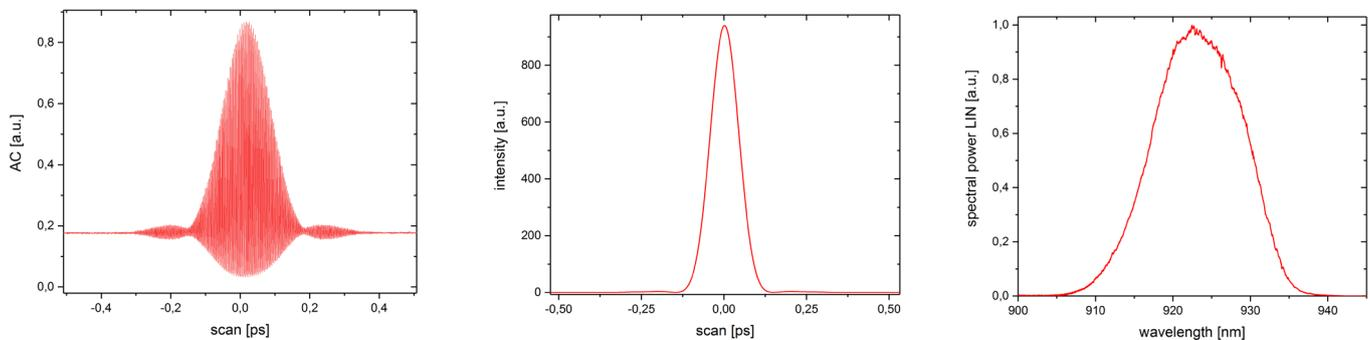
Figure 1: Test results of the new FemtoFiber ultra 920. Autocorrelation trace and retrieved pulse shape of the FemtoFiber ultra 920 feature <100 fs pulses with 99% of the laser power within the main pulse. The emission spectrum is centered at ~920 nm with a bandwidth of ~15 nm and emission spectrum.
