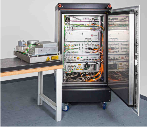
Fig. 1: Photograph of the laser system consisting of a laser head and an electronics cabinet. On the left: Laser head with Raman fiber amplifier (RFA) and second-harmonic generation (SHG) modules installed on a water-cooled cold plate on top of a stainless steel frame. The interface (fiber-optical, electrical and coolant connections) is on the rear side. The thermal and protection shields have been removed. On the right: The cabinet with external and coolant interfaces on the bottom and laser head interface on the top.
