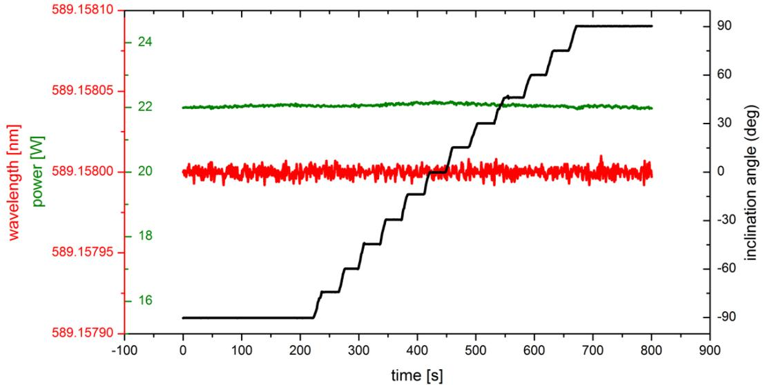
Fig. 6: Output power and emission wavelength of the laser with varying inclination angles of the laser head.
