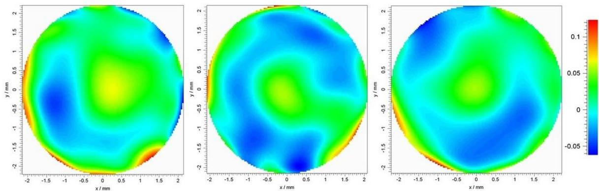
Fig. 5: The above plot shows the wavefront quality measured with a Shack-Hartmann wavefront sensor over  $\sqrt{2}$  times the beam diameter (3 mm). The scale on the right shows the color code of the wavefront error in waves
