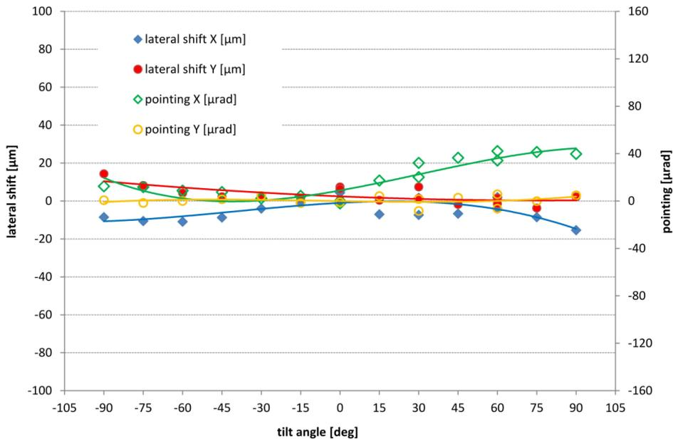
Fig. 7: Lateral shift and pointing of the laser beam under varying gravity conditions using a tilt test stand and the ESO BCDS unit.
