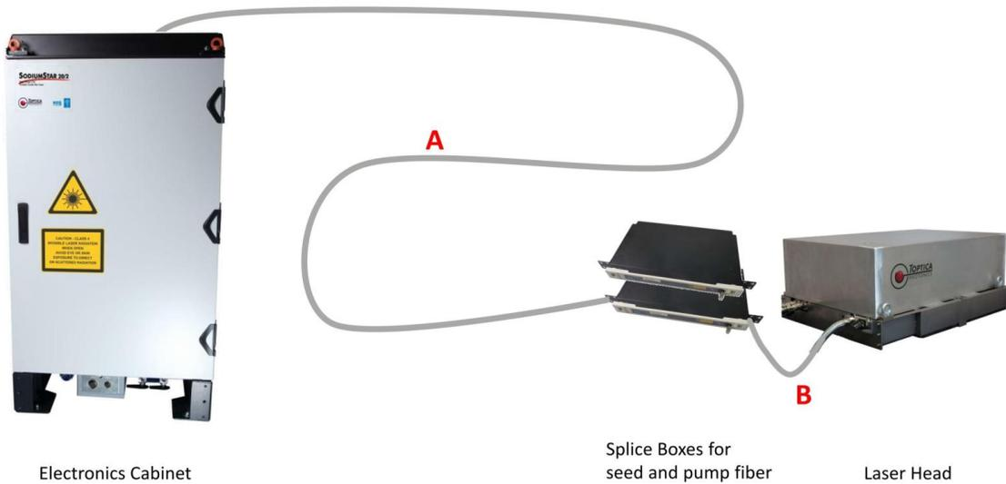
Fig. 2: Remote pumping configuration as used for the W. M. Keck telescope. The distance between LH and EC is 27 m (fiber length A + B). Two splice boxes for the seed and pump fibers are located close to the LH.
