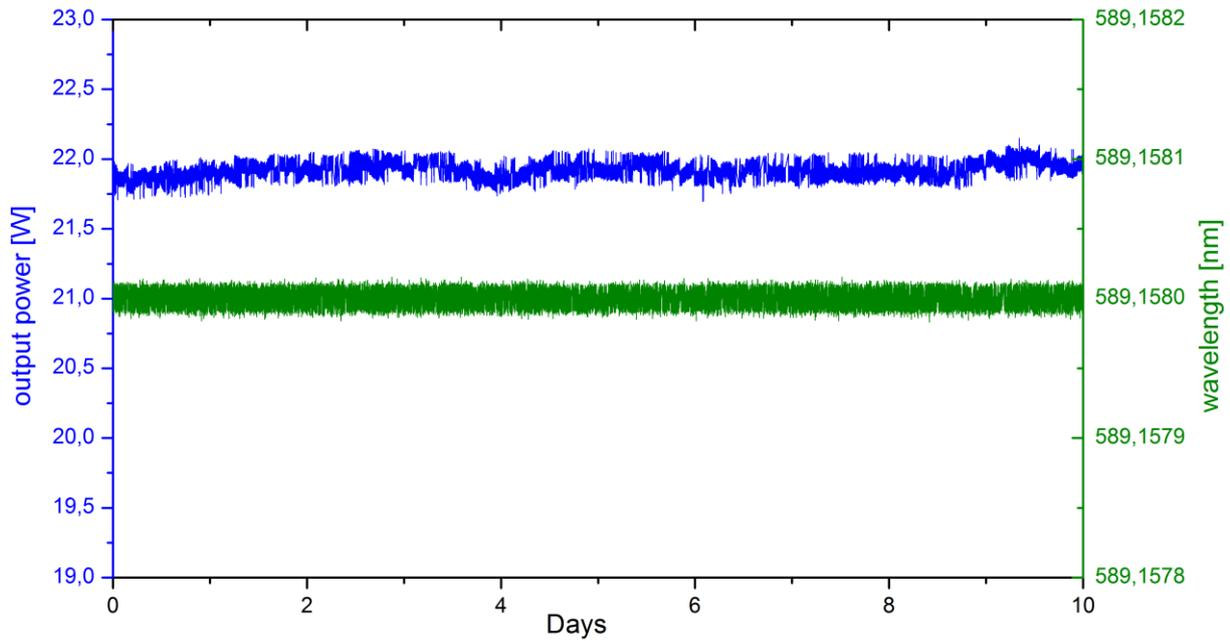
Fig. 4: Output power and wavelength measurement of laser unit SN #6 over a period of 10 days showing excellent stability without any long-term drifts.
