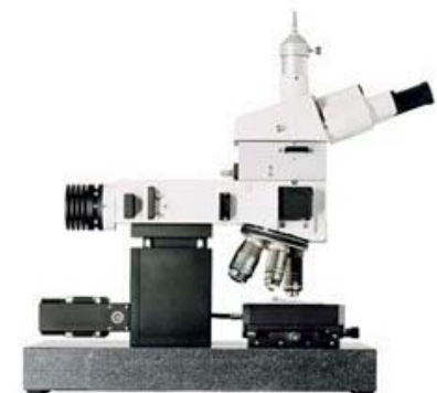
Picture 9: Modern Confocal Raman Imaging Microscope WITec alpha300 R. Courtesy of WITec.
