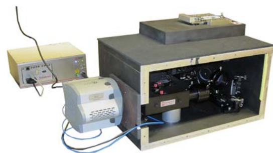
Fig. 2: Custom-built TIRF microscope with EMCCD camera and iChrome MLE.
