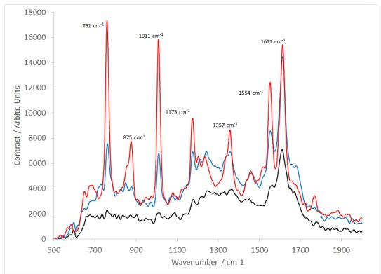
Fig 5. Raman spectra of IgG (30 second integration time, average of 10 frames). Solid black line: IgG is measured in static configuration; Blue line: IgG measured with sample rotating during the observation; Red line: IgG measured with a complex motion applied using a rotation and linear stage
