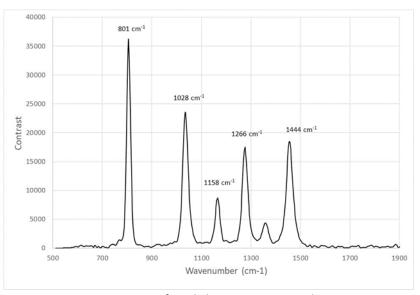
Fig 4. Raman spectrum of cyclohexane captured in 1s
