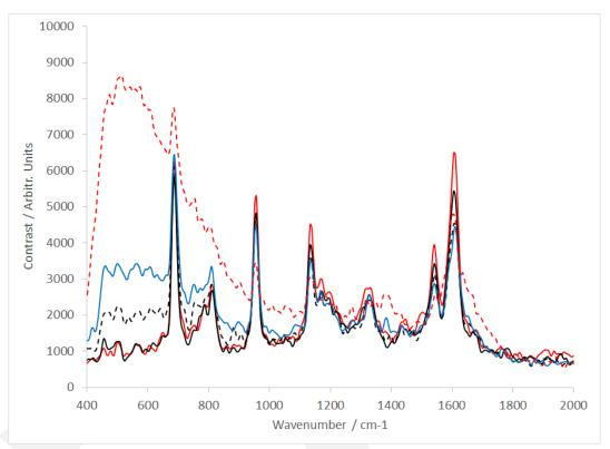
Fig 10. Raman spectra of dAb (sample provided by the TESTA centre, Cytiva Life Sciences) of different concentration levels: dotted red line =  $0.1 \, \text{mg/ml}$ , solid blue line =  $0.5 \, \text{mg/ml}$ , dotted black line =  $1 \, \text{mg/ml}$ , solid black line =  $5 \, \text{mg/ml}$  and solid red line =  $10 \, \text{mg/ml}$
