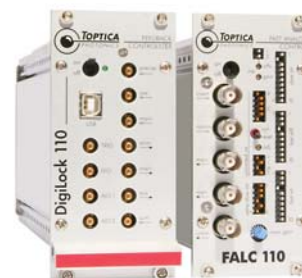
Fig. 5: DigiLock 110 and FALC 110: modules for linewidth narrowing.
