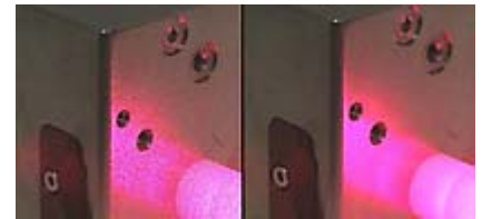
"Speckle killer": the speckle pattern in the left image is eliminated by electronic means (right).
