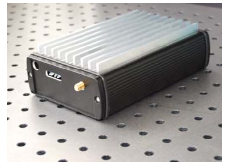
Laser coherence control unit LCC: linewidth broadening up to GHz ranges.
