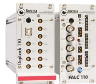
DigiLock 110 and FALC 110: modules for linewidth narrowing.
