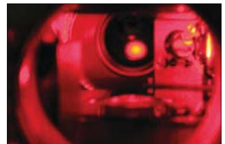
Magneto-optical trap of lithium atoms. T. Esslinger, ETH Zürich, Switzerland.
