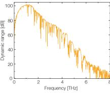
Time-domain terahertz spectrum (dynamic range of terahertz power), measured with TOPTICA's TeraFlash pro. All of the dips are absorption lines of water vapor.
