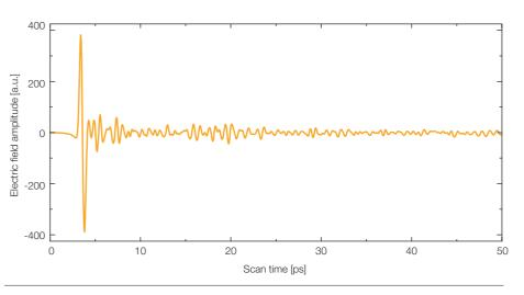
Pulse trace of an InGaAs photoconductive switch.
