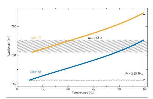
Frequency calibration of a TeraBeam 780 system. The wavelengths of the two DFB lasers overlap at approx. 784.6 nm (shaded bar). By heating laser #1 and cooling laser #2, the difference frequency increases up to 2.3 THz.
