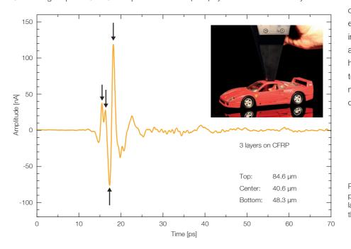
test, and fail in case of non-metallic substrates. Terahertz pulses, by contrast, resolve the thickness of each individual layer, as long as adjacent coatings differ in their refractive index.
