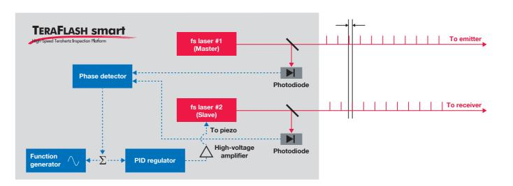
Schematic diagram of the TeraFlash smart. Blue lines depict electric signals, red lines the optical signals. The black arrows depict the momentary difference in repetition rates.
