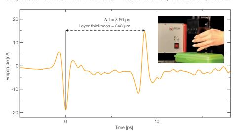
multi-layered samples, via time-of-flight techniques: Each layer interface reflects a part of the incident pulse, and the time elapsed between the arrivals of pulse "echoes" from either side is directly proportional to the optical thickness of that layer.
