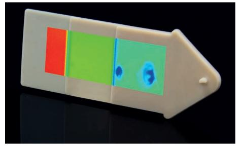
The liquid state of water generally provides a stark contrast in terahertz imaging - a property exploited in humidity measurements in paper production lines. Water contrast terahertz imaging can help to avoid drought stress and optimize irriga-
