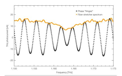
Terahertz scan across a water-vapor resonance. The black trace depicts the phase "fringes" as measured with a TeraScan 1550 system. The yellow trace shows the envelope spectrum obtained with the Phase Modulation Extension; the high frequency resolution unveils small-scale standing-wave effects in the optical path.
