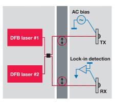
Schematic of TeraScan with Phase Modulation Extension (dark grey).
