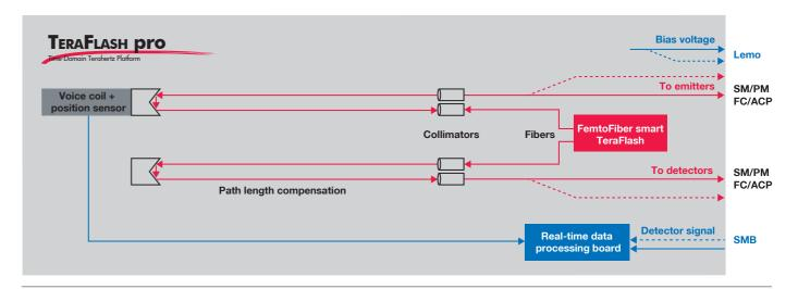
Schematic diagram of the TeraFlash pro. Blue lines depict electric signals, red lines the optical signals.
