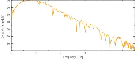
Terahertz spectrum of air with water vapor lines, obtained with the TeraFlash smart. With 1000 averages, the spectrum spans almost 5 THz – within a measurement time as short as 600 milliseconds.
