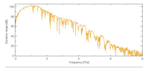
Terahertz spectrum of air with water vapor lines, measured with the TeraFlash pro. Within a measurement time of less than half a minute, the bandwidth reaches 6 THz and the peak dynamic range exceeds 95 dB – an industry record!
