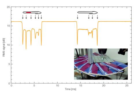
1D-scan of folded cardboard boxes with and without a package slip. The graph shows the transmitted terahertz intensity while the boxes moved at a velocity of 21 m/s. In the example, the TeraSpeed recorded more than 150,000 intensity values per second.
