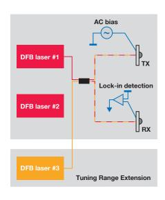
Schematic of TeraScan (red) with Tuning Range Extension (yellow).
