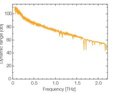
Frequency-domain terahertz spectrum (dynamic range of terahertz power), measured with TOPTICA's TeraScan 1550 (+ Tuning Range Extension 2.0).
