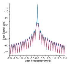
Measurement of the CTL 950 linewidth with a self-heterodyne beat experiment with a 1 km (5 µs) delay fiber. The result is a linewidth of approximately 5 kHz.
