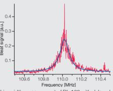
Linewidth measurement of DL 100 with delayed self-heterodyne beat setup (delay 5 µs). The resulting linewidth is below 100 kHz.
