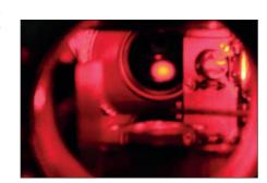
Magneto-optical trap of lithium atoms. T. Esslinger, ETH Zürich, Switzerland.
