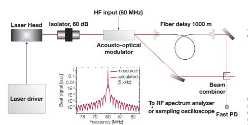
Delayed self-heterodyne linewidth measurement and typical result.
