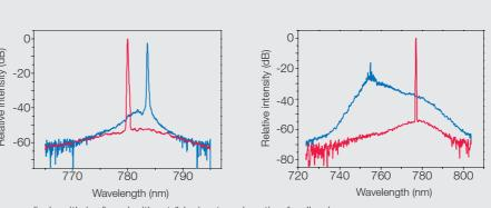
Laser diode with (red) and without (blue) external grating feedback. The left graph shows an FP diode, the right graph an AR diode.
