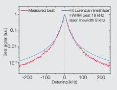
Measured beat signal of two free-running DL pro at 1160 nm. 100 scans with sweep times of 50 ms have been averaged. The two laser systems are of the same built and contribute equally to the residual noise.
