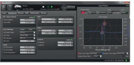
Convenient laser control via remote PCoperation: Users can easily set all relevant parameters via the graphical user interface.
