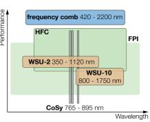
Comparison of frequency references. The performance represents aspects like accuracy, repeatability or achievable linewidth. Shown are: Frequency comb (DFC) wavelength meters (WSU), spectroscopy cells (CoSy), Fabry-Pérot interferometers (FPI), and high finesse cavities (HFC).
