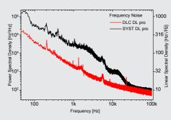
**Right:** Frequency noise density of the laser light created with a DLC DL pro and a SYST DL pro.
