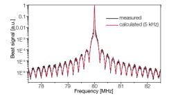
Self-heterodyne linewidth measurement of DLC DL pro with narrow linewidth option.
