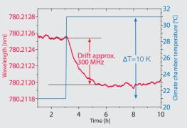
Laser frequency response to a 10 Kelvin air temperature change (laser and electronics inside a climate chamber).
