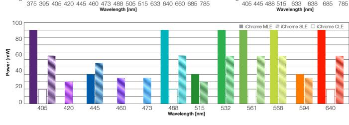
Output power/wavelength chart of TOPTICA's single-mode (top left) and single-frequency (top right) diode lasers as well as multi-laser engines (bottom).
