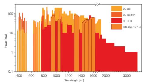
diodes. It offers larger mode-hop-free tuning ranges at reduced coarse-tuning ranges and increased linewidth compared to the DL pro. Due to the lack of alignment sensitive optical elements, DFB pro lasers are suited particularly for applications in noisy environments.
