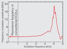
DL pro piezo transfer function. Below 4 kHz no acoustic resonances can be detected.
