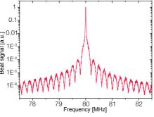
A self-heterodyne linewidth measurement shows a short-term linewidth of a free-running DLC DL pro (narrow linewidth option) of only
