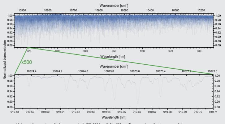
High resolution spectrum of iodine measured with CTL 950 from 915 to 985 nm. The zoom shows the immense resolution. With piezo scanning more than two additional x500 zooms are possible to measure even finer features and resonances.
