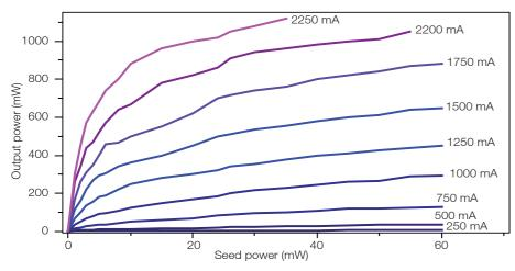
Typical saturation behavior of tapered amplifier chips at different amplifier currents (seed power levels exceeding 40 mW are not recommended).
