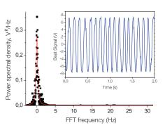
Beat measurement of two independent ECDLs locked to two high-finesse ULF cavities, one of them using FALC 110. The beat width was less than 0.5 Hz over 8 s. The inset shows the phase stability of the beat note filtered with a 100 Hz low-pass filter (J. Alnis, MPQ Garching).
