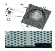
Another important application for CTLs are quantum dots. These act as artificial atoms in in solid-state systems. Unlike real atoms, semiconductor quantum dots can be grown and placed in a controlled fashion, e.g. in photonic crystal cavities and even enable cavity QED experiments in the solid state (taken with permission from Peter Lodahl et al., Reviews of modern physics 87, p. 347 (2015)).
