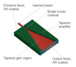
Geometry of a tapered amplifier chip.
