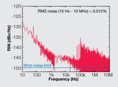
Relative intensity noise (RIN) of a DFB pro laser at 780 nm. The integrated RMS noise amounts
