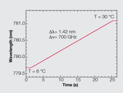
"Wide scan" of a DFB pro laser at 780 nm: A temperature sweep from 3 °C to 30 °C changes the frequency by 700 GHz.
