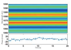
Typical result of spectral interferometry for out-of-loop measurement of the CEP stability.
