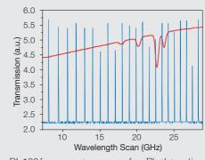
DL 100 frequency sweep over four Rb absorption FSR 1 GHz) are shown for reference.
