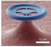
The CTL is ideally suited to investigate microcavites. Such cavities are useful for sensing applications, investigating quantum-mechanical coupling, and to create microscopic frequency combs.
