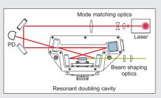
Schematic of SHG pro, stand-alone resonant frequency-doubling cavity.
