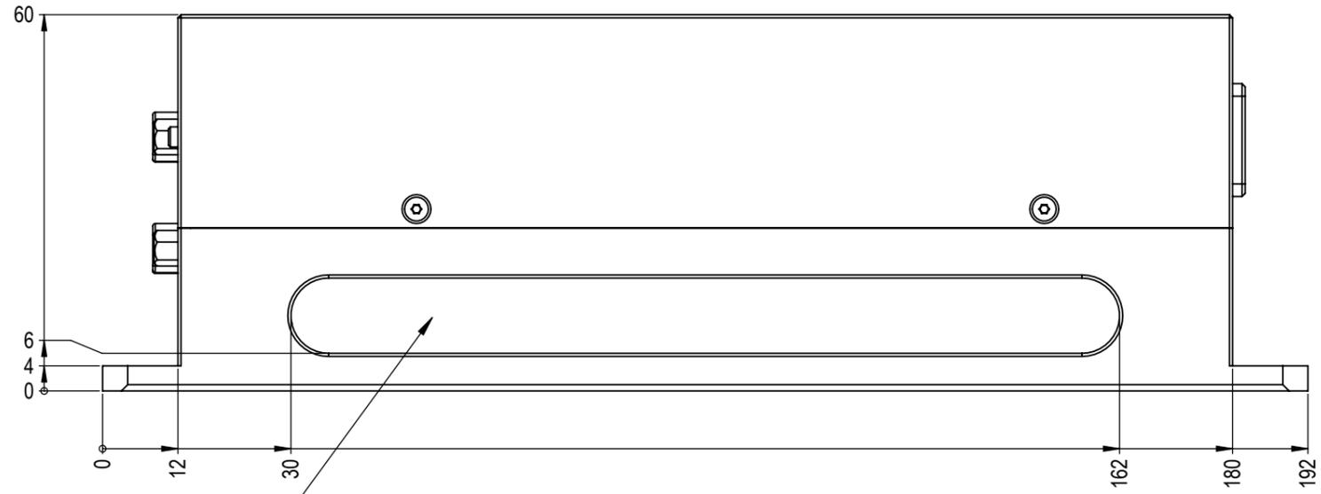
channel for mounting clamps: depth 3mm
