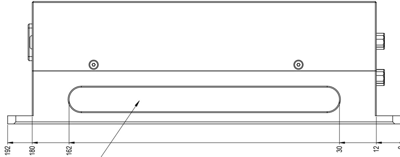
channel for mounting clamps: depth 3mm
