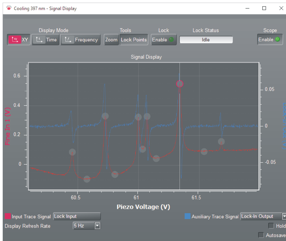
Figure 63 Signal Display showing the Lock Input signal (Input Trace Signal, red) and the Lock-In Output signal (Auxiliary Trace Signal, blue) for Top of Fringe locking and lockpoint candidates (example)
