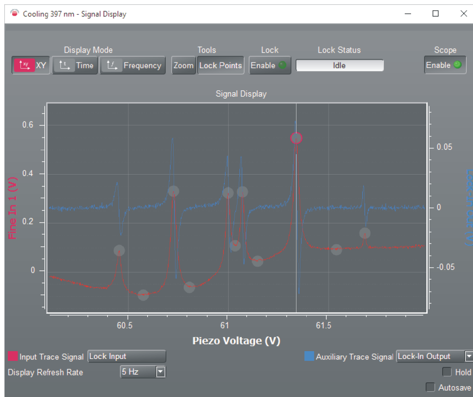
Figure 63 Signal Display showing the Lock Input signal (Input Trace Signal, red) and the Lock-In Output signal (Auxiliary Trace Signal, blue) for Top of Fringe locking and lockpoint candidates (example)
