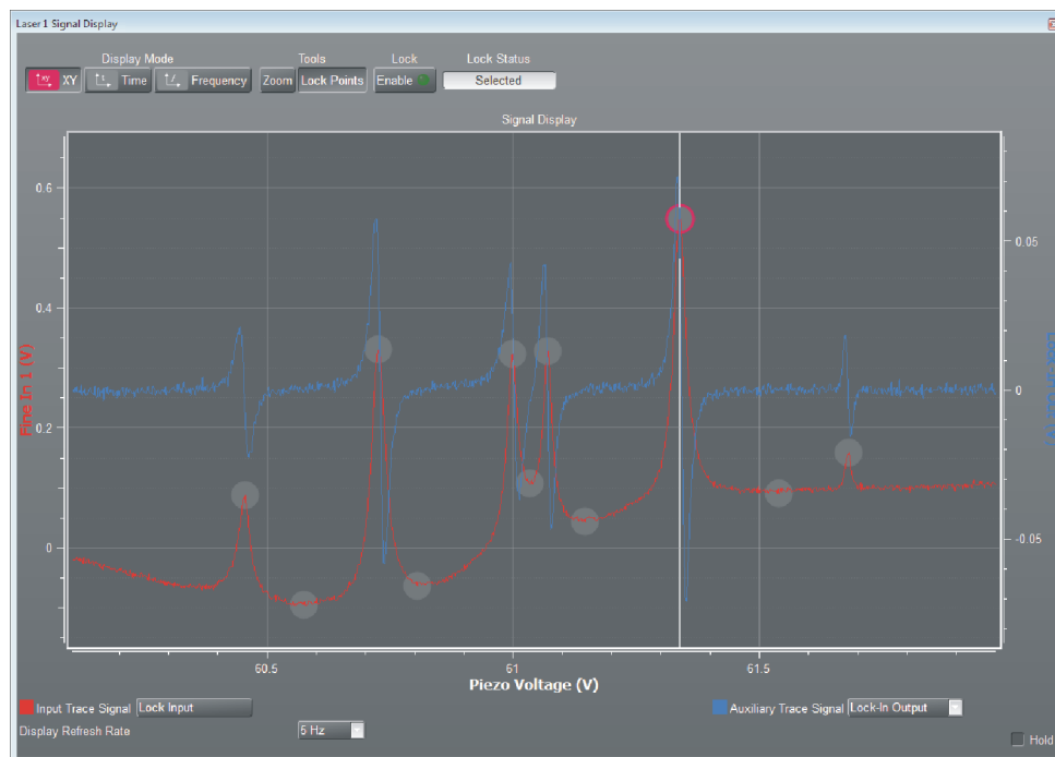
Figure 73 Signal Display showing the Lock Input signal (Input Trace Signal, red) and the Lock-In Output signal (Auxiliary Trace Signal, blue) for Top of Fringe locking and lockpoint candidates (example)
