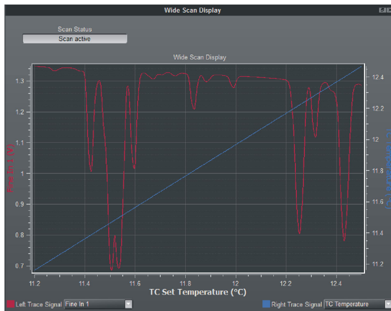
Figure 76 Wide Scan Display showing a molecular absorption spectrum (left/red curve) and the TC Temperature signal (right/blue curve)
