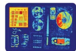
Photograph (top) and terahertz image (bottom) of a suitcase with various objects (courtesy Synview GmbH).
