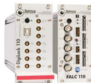
DigiLock 110 and FALC 110: modules for linewidth narrowing.
